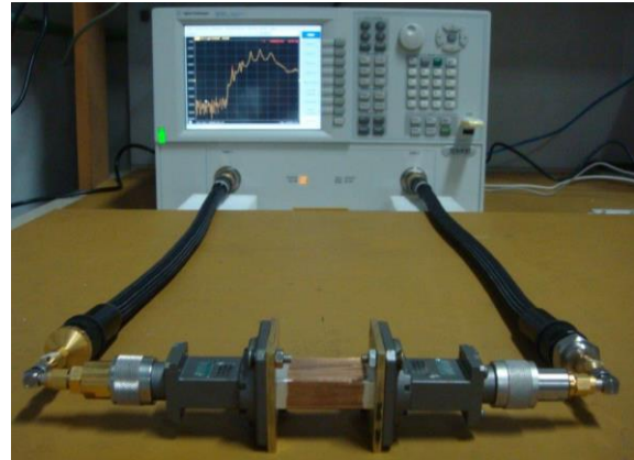
Fig. 5. Setup to measure the transmission and reflection bands of the loaded waveguide.
