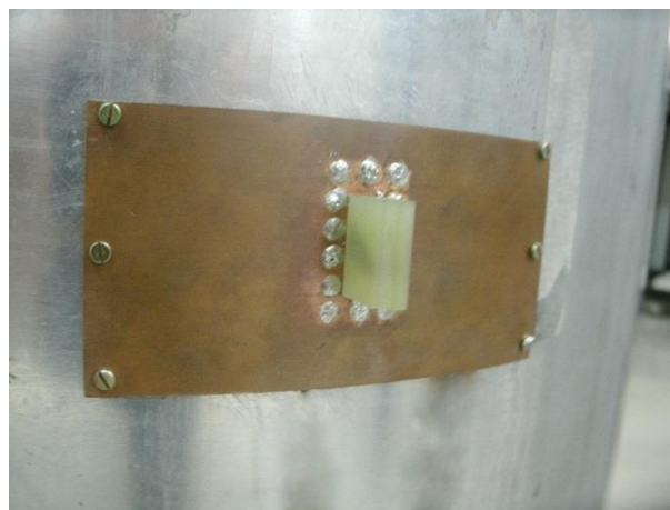
Fig. 19. Prototype of blade antenna on metallic cylinder.
