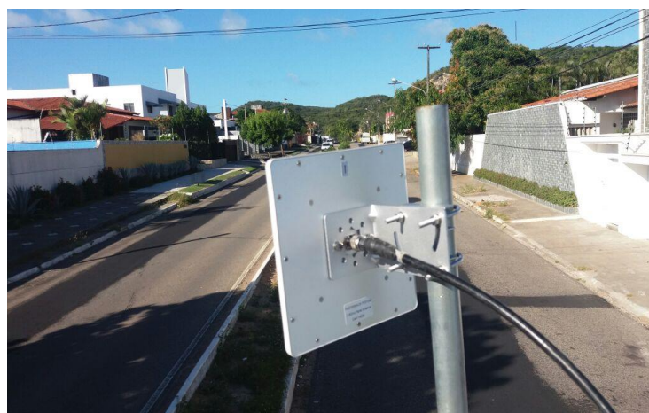
Fig. 1. One of the streets from Lagoa Nova district, highlighting the panel antenna used in reception.
