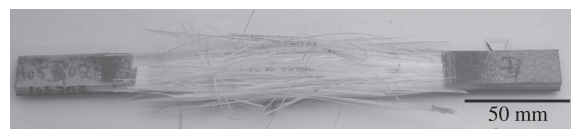
Figure 14. Photograph of GFRP samples that failed under tension.
