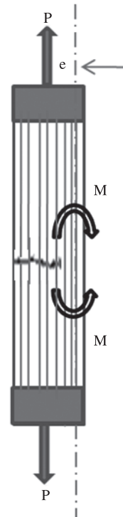
Figure 13. Schematic of state of stress during final fracture region in a composite specimen that failed under tensile load.
