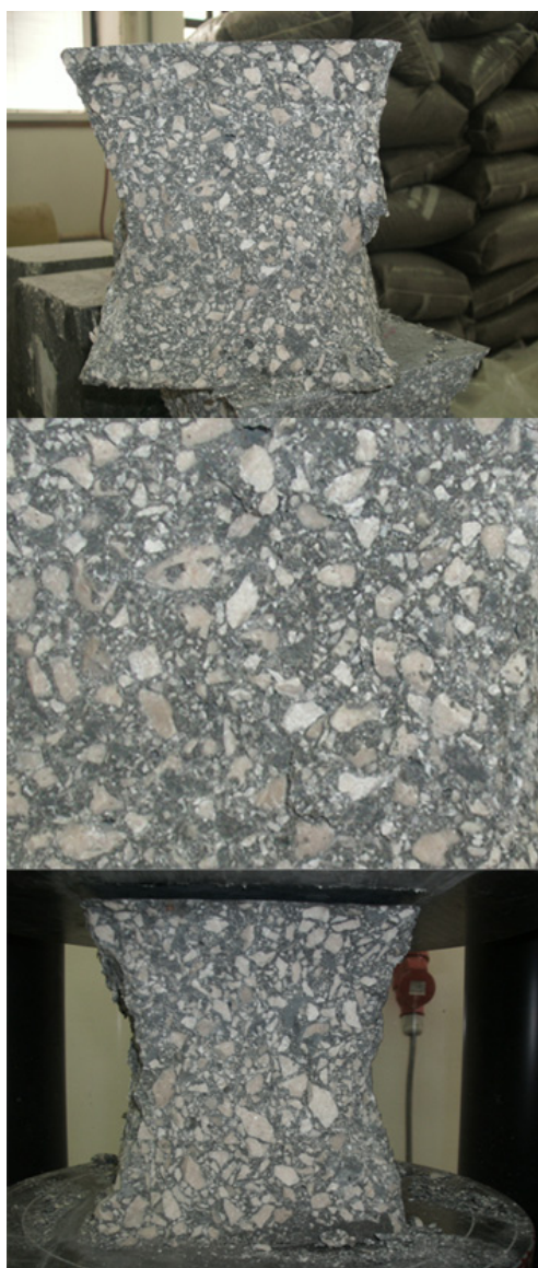
Figure 12. ESCC, MSCC and VSCC specimens after compressive strength tests.
