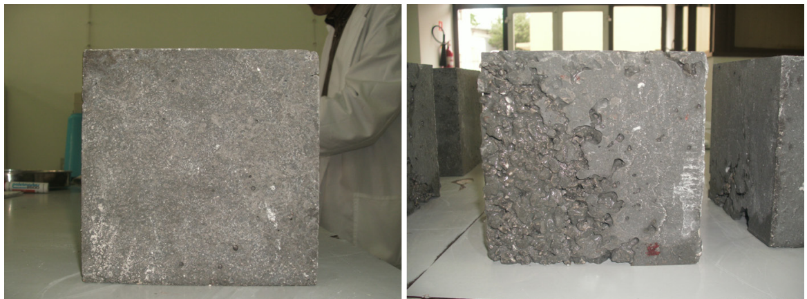
Figure 9. The appearance of the surface of ESCC samples - two samples (good - left, bad - right).
