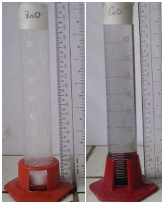
Figure 3. Stability of ZnO and CuO in acetone.
