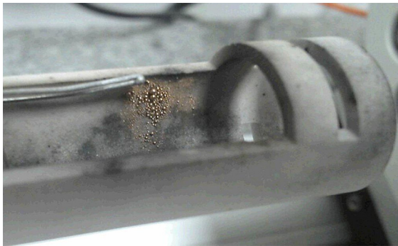
Figure 2. Vaporization of copper inside the dilatometer tube.
