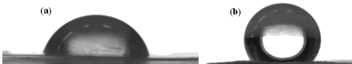
Figure 10. Shape of water drop on the air side of: (a) PHB film ( \theta=77.10^\circ ) and (b) PHB nanofibers mat ( \theta=130.30^\circ ).
