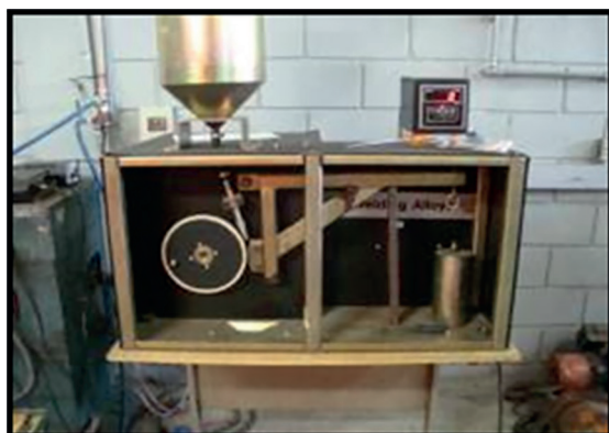
Figure 3: Rubber wheel abrasion resistance machine used to simulating the low stress abrasion.
