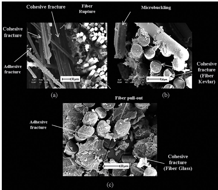
Figure 13. Fracture characteristics – HFCL laminate.
