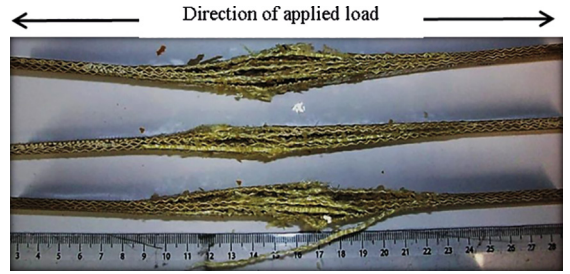
Figure 7. Fracture characteristic - HFCL laminate - uniaxial tensile.
