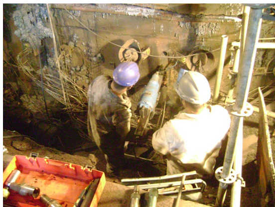
Figure 2. Drilling the furnace metal shell to collect the drill core sample.
