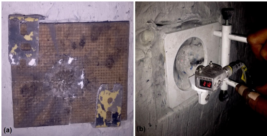
Figure 4. (a) Indentation depth in the clay witness caused by the bullet impact on MAS after ballistic impact. (b) Measurement with Laser sensor caliper, model Q4X by Banner manufacturer.
