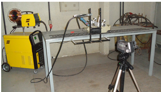
Figure 6. Experimental bench for IR measurements. The infrared images were recorded on the backside of the absorbing part
