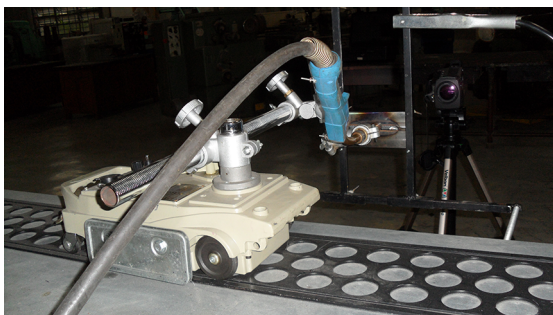
Figure 1. Automated GMAW process utilized in this work
