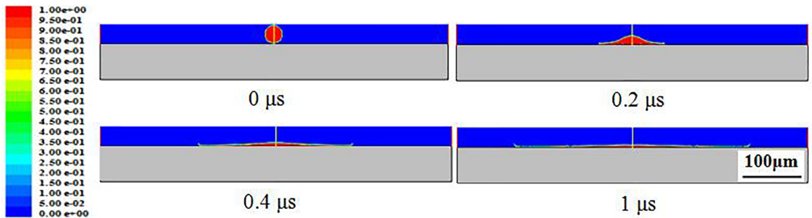
Figure 7. Changes of a droplet deformation and solidification with time for Ø50 \mu\text{m} and 200 m/s
