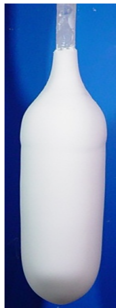
Figure 2. Green body formed by agglomerated silica nanoparticles synthesized by VAD.
