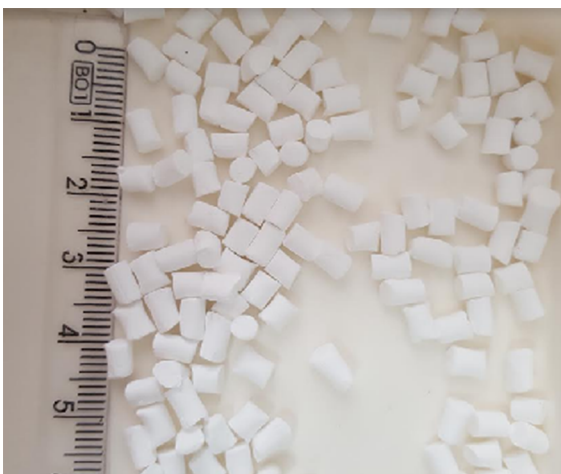
Figure 4. Final SBA-15 extrudates calcined at 800 °C.
