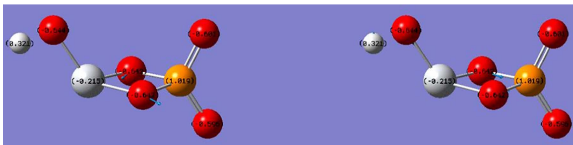
Figure 7. Stationary geometry of Ti (II) interaction with oxygen in the complex [\text{Ti}(\text{OH})\text{PO}_4]^{2+} (Ti - larger grey atom, O - red atom, P - orange atom, H - smaller grey atom) (a) antisymmetric centralized oscillation (b) symmetric centralized oscillation; quasi-chair structure , which is a favorable structure.
