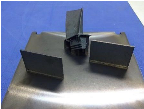
Figure 2. Samples of vertically built specimen in DMLS.
