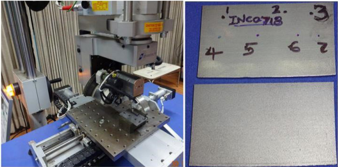
Figure 3. XRD Residual Stress Measurement.
