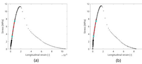
**Figure 12.** Maximum stress (*i.e.*, at the bottom of the beam) as the respective longitudinal strain for the (a) front and (b) back analyzed surfaces. The cyan circles depict the points used for calculating the Young's modulus (the same points are highlighted in Figure 10(b)), and the respective affine slope is shown as a dashed red line.
