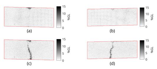
Figure 14. Absolute gray level residuals normalized by the dynamic range of the reference images for (a, b) the ultimate load and for (c,d) the last frame. Results for the front surface in sub-figures (a,c) and for the back surface in sub-figures (b,d).
