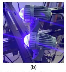
Figure 6. (a) Effect of the blue bandpass filter on image acquisition at 900°C. (b) 10W blue LED illumination dedicated to one of the furnace windows.
