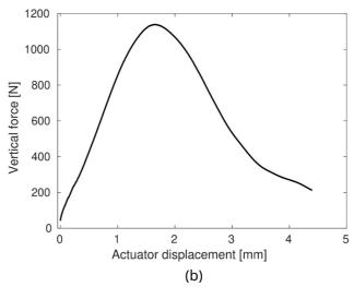
Figure 15. (a) Post-mortem wedge splitting test sample inside the F900 furnace. (b) Loading curve obtained with the 900°C setup.
