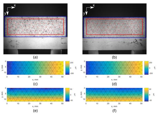
Figure 8. (a,b) References images with the meshes (in red) used for analyzing the YSZ specimen dilatometry up to 850°C. (c,d) Horizontal and (e,f) vertical displacement fields for the maximum temperature. Sub-figures for the front face in (a,c,e) and for the back face in (b,d,f). In the images,  $1 \text{ px} \approx 13.4 \text{ }\mu\text{m}$ .
