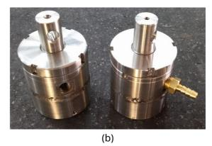
Figure 4. (a) CAD project of the coupling/cooling parts for the actuators and (b) the final parts in stainless steel. See "cooling of actuators" in Figure 2 for visualizing these parts in the setup.
