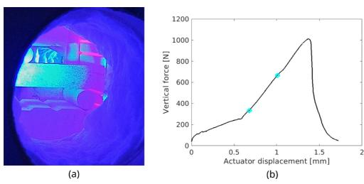
Figure 10. (a) Three-point bending sample inside the F900 furnace at 900°C during the experiment. (b) Resulting loading curve. The cyan circles depict the region where the Young's modulus was calculated.
