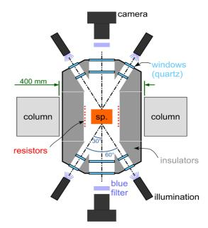
**Figure 1.** Top view of the furnace for up to 900°C tests displaying the setup used in the analyses presented in Section 3.
