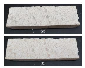
**Figure 7.** Silicon carbide slurry pattern of a parallelepipedic sample (of approximately  $10 \times 25 \times 120 \text{ mm}^3$ ) made of the same material used in three-point bending (Section 3.2) and WST (Section 3.3) (a) before and (b) after being heated up to 900°C.
