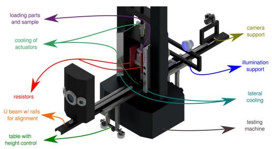
Figure 2. 3D assembly of the developed F900 setup to perform thermomechanical experiments up to 900°C.
