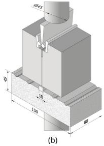
Figure 5. 900°C setups for (a) bend experiments and (b) WSTs. Dimensions are given in mm.
