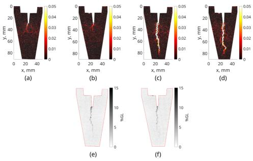
Figure 18. Maximum principal strains for (a,b) the time step of the ultimate force and (c,d) for the last time step of the WST performed at 900°C. (e,f) Absolute gray level residuals for the last analyzed time step normalized by the dynamic range of the reference images. Results for the front surface in sub-figures (a,c,e) and for the back surface in sub-figures (b,d,f).
