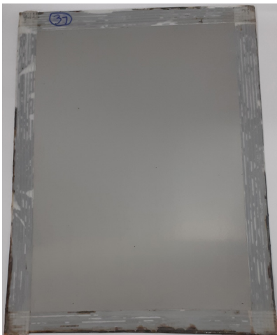
Figure 5. Photograph of a representative panel of specimen 4 EP-ET, after 47 days of exposure in the humid chamber test. The abbreviation EP-ET means electrolytic pickling and electrolytic chemical treatment respectively.
