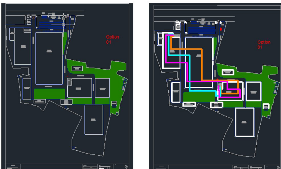
Figure 3. Current Plant Layout and Spaghetti Diagram. Note: The orange line represents the circular loom flow, the green line represents the needle loom flow, and the pink line represents the flat loom flow.
