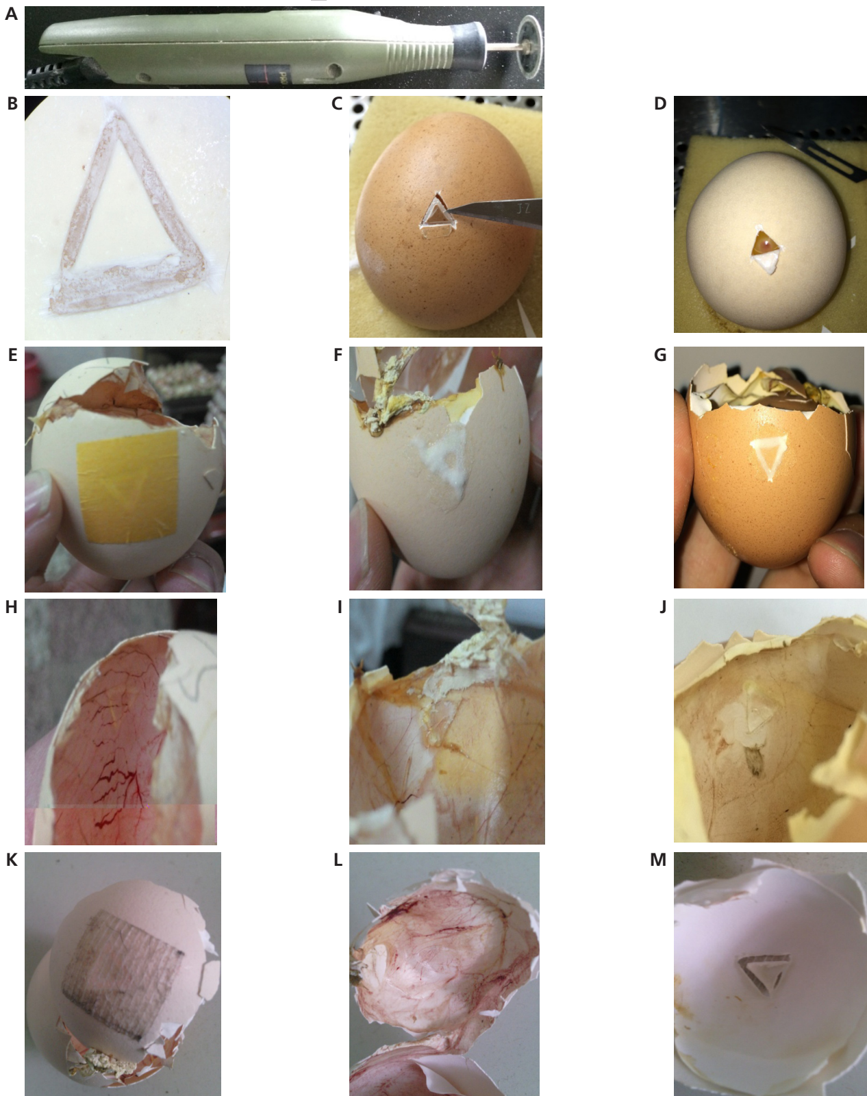
Figure 1 – A: Egg shell cutting tool. B: The triangle groove, only cutting the outer shell without destroying the inner shell membrane, the width of one side was two times the width of the other two. C: 2 mm 2 double faced adhesive tape was glued beside the wider seam, and the inner membrane of the other two seams of the triangle cover can turn over along the wider seam. D: After opening the shell and injecting DMEM into the embryo, a red spot was apparent in the middle of the embryo. E: The outside part of the window sealed with the SBT (yellow sticky paper tape, 3M 244, Scotch Brand Tape). F: The outside part of the window sealed with "SP+IG" (Straw powder, FHK, Japan, was firstly sprinkled on the groove evenly, then one or two drops of instant glue, 502, super glue, China, were dropped spreading along the whole grooves. G: The window sealed with IG first, then sprinkled with SP. H: After hatching, the internal part of the window sealed with SBT. I: After hatching, the internal part of the window sealed with SP first, then dripped with IG. J: After hatching, the internal part of the window that was sealed firstly with the IG, then sprinkled with SP. K: The blunt end window sealed with SST (the medical sterile sticky tape with side of 1.2x1.5 cm, Steri-Strip™, American). L: After hatching, the punctured part of the inner membrane under the window being sealed with SST in the blunt end. M: After hatching and the inner membrane being removed, the internal part of the window which was sealed with SST in the blunt end.
