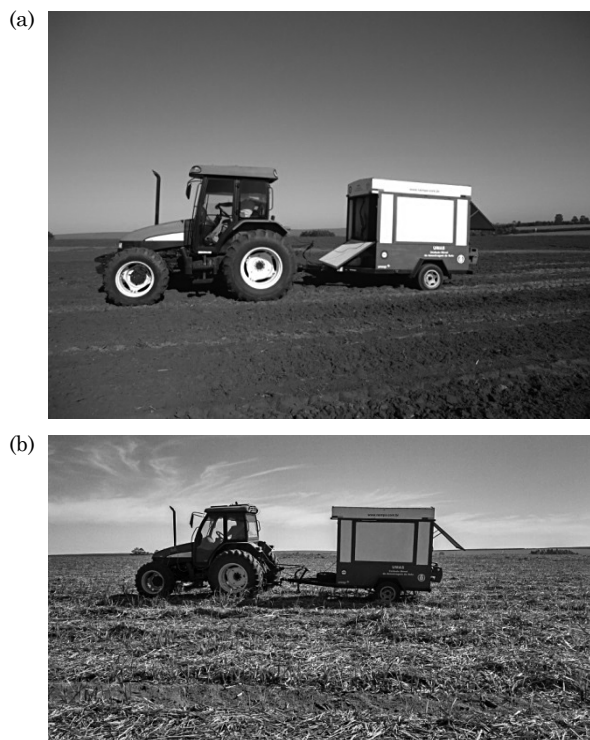
Figure 2. Evaluation after soil tillage (a) and after sugarcane harvest after 15 months (b) with the mobile soil sampling unit.
