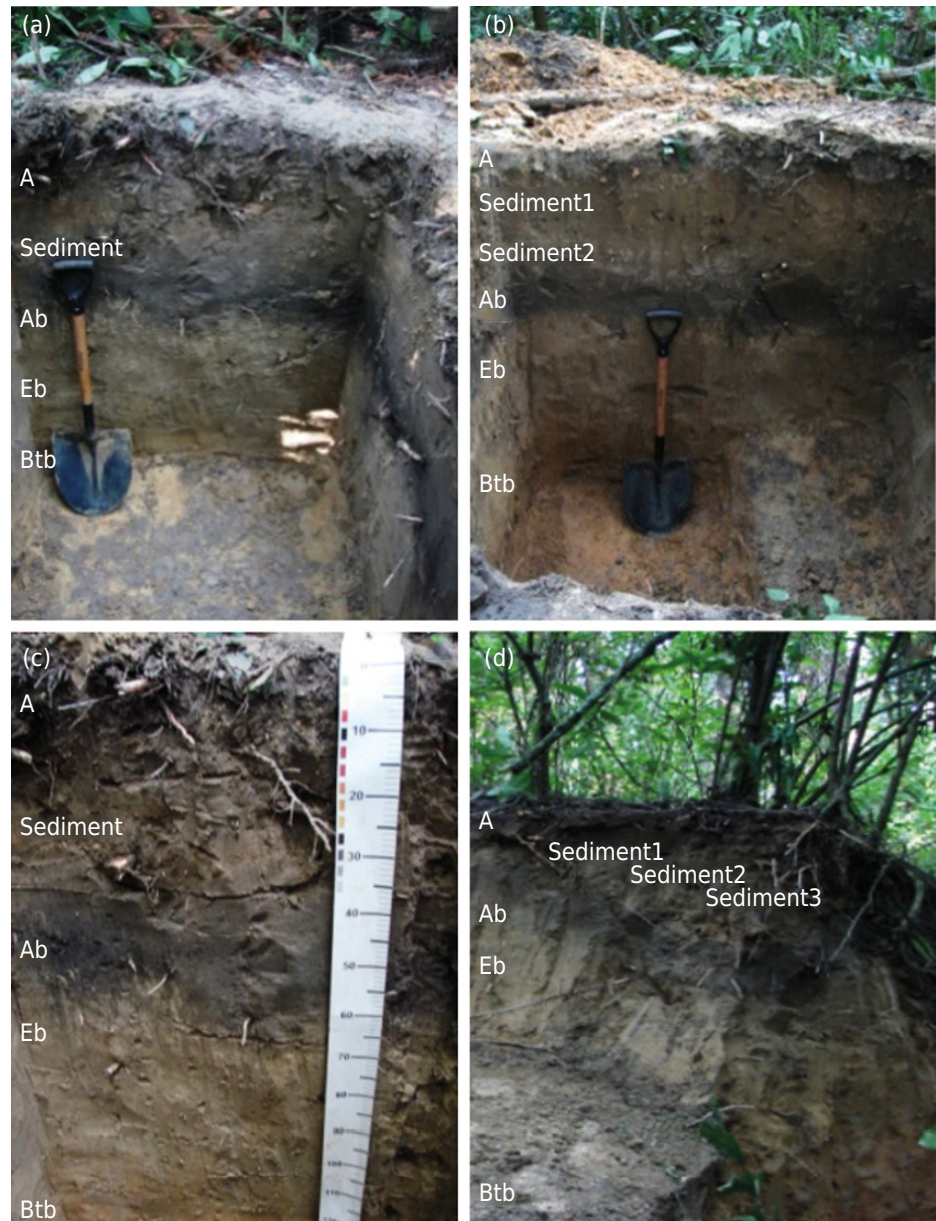
Figure 2. Images of the studied pits: soil horizons and sediment layers. (a) Pit 1 - T1; (b) Pit 2 - T2; (c) Profile 1 - P1; and (d) Profile 2 - P2.
