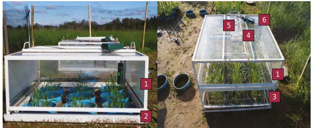
Figure 1. Labeling chamber used for in situ ^{13}\text{C} pulse labeling. Components are: (1) labeling chamber, (2) galvanized steel base, (3) chamber extension, (4) fan, (5) rubber septum and plastic container (inside) for ^{13}\text{CO}_2 production, and (6) IRGA.
