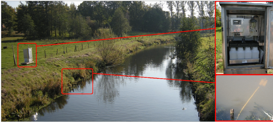
Figure 2. Automatic water sampler MAXX SP III® installed at the gauge station Willenscharen, Germany
