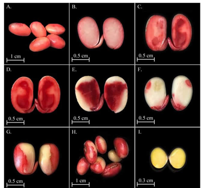
Figure 2. Separation and classification of soybean seeds subjected to tetrazolium test. (A) normal seeds; (B) normal seeds without damage to cotyledons and embryo; (C) normal seeds with lesions in the cotyledons; (D) normal seeds with lesions in the cotyledons and embryo; (E) seeds injured in the coat with damage to the cotyledons and embryo; (F) injured seeds without respiratory activity in the cotyledons and injured embryo; (G) seeds injured in the coat; (H) injured seeds; (I) hard seed
