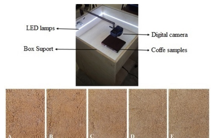
Figure 1. Image acquisition system and coffee samples in five impurities percentages: 0 (A), 10 (B), 30 (C), 50 (D) and 70% (E)
