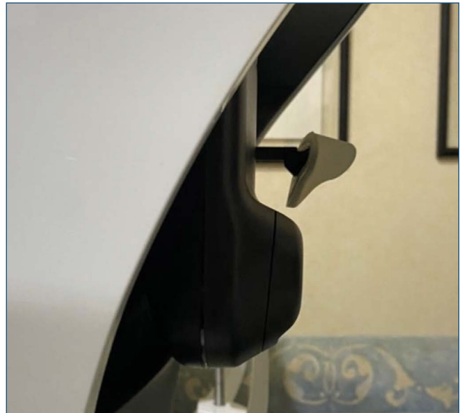
Figure 3. Maximum forehead adjustment on Essilor phoropter Vision-S™ 700.
