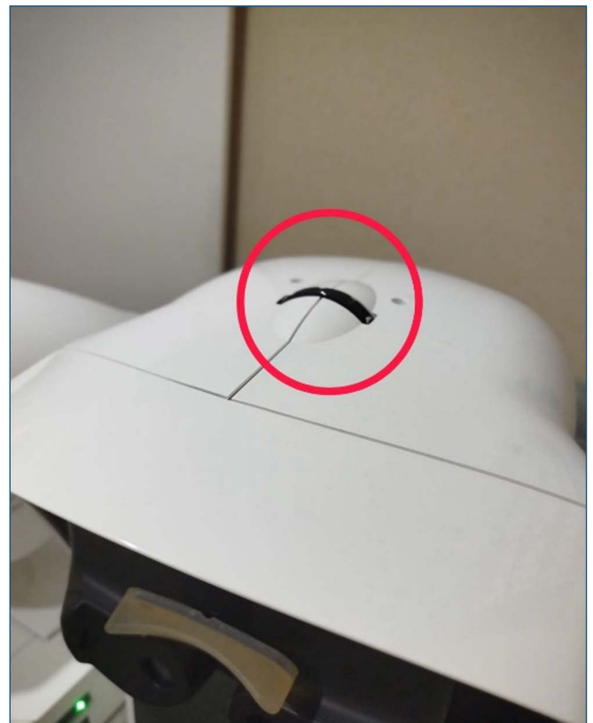
Figure 1. Vertex distance adjustment Knob of Essilor phoropter Vision-S™ 700.
