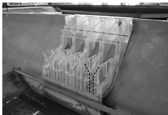
Figure 9. “Y” shaped Slit Bucket structure (Alternative 7).
