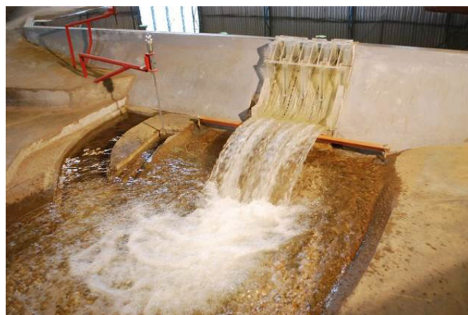
Figure 6. Pilot hydraulic model used in tests – original configuration.
