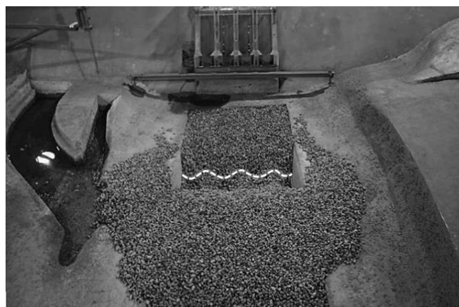
Figure 15. Scour hole formed in the test of Alternative 3 for a flow with a 5-year recurrence.
