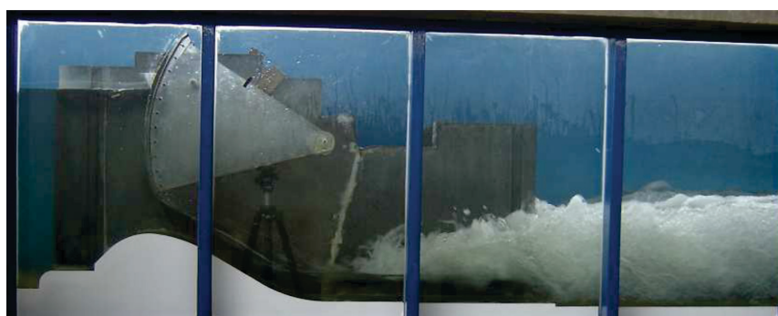
Figure 2. Hydraulic jump formed for flowrate 227 l/s and incident Froude number 3.69.
