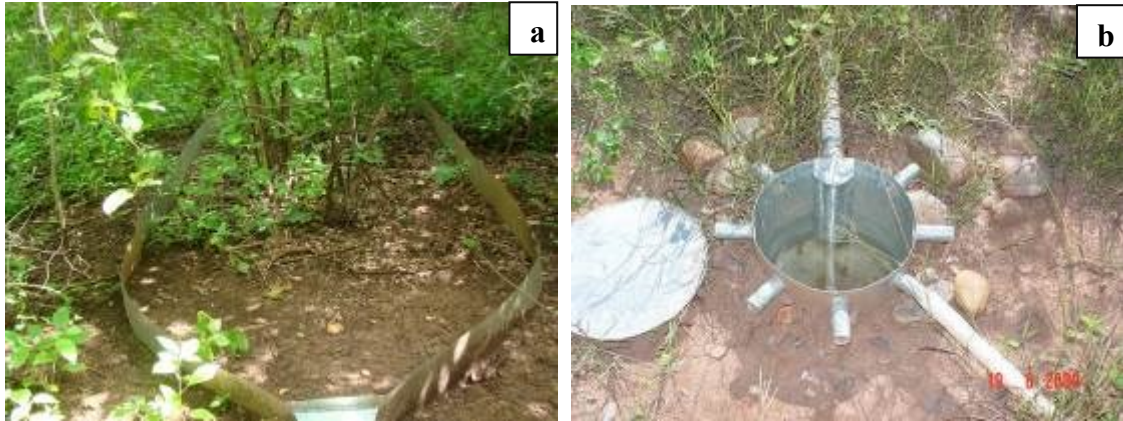
Figure 3. Plot of 20 m 2 (a) installed in the experimental watershed with a typical caatinga vegetation cover with regeneration for over 35 years, from the Iguatu Experimental Basin (IEB); first collector tank (b).
