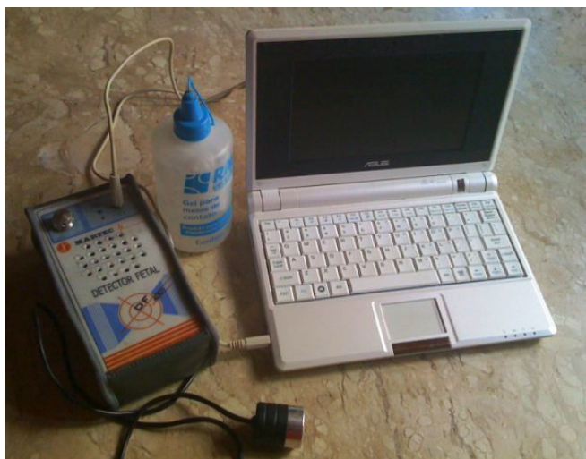
Figure 1. Doppler sonar coupled to a computer and the contact gel
