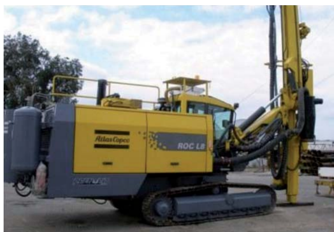
Figure 4 Atlas Copco ROC L8 drill rig.
