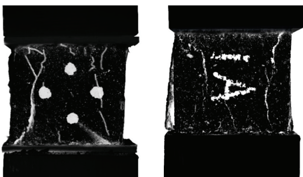
Figure 14 Formation of conical cracks for l/h = 1.0
