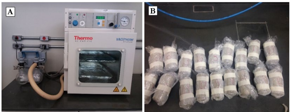
Figure 1. Stages of the precondition adopted: 1 st Stage - vacuum oven (A) and 2 nd Stage – Samples packaged in a plastic film (B).
