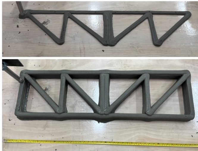
Figure 13. Example of a lattice specimen printed with Mix A.
