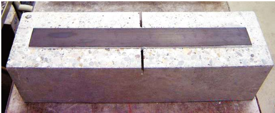
Figure 7 - Notched concrete beam post-strengthened with the Sika® Carbodur system
