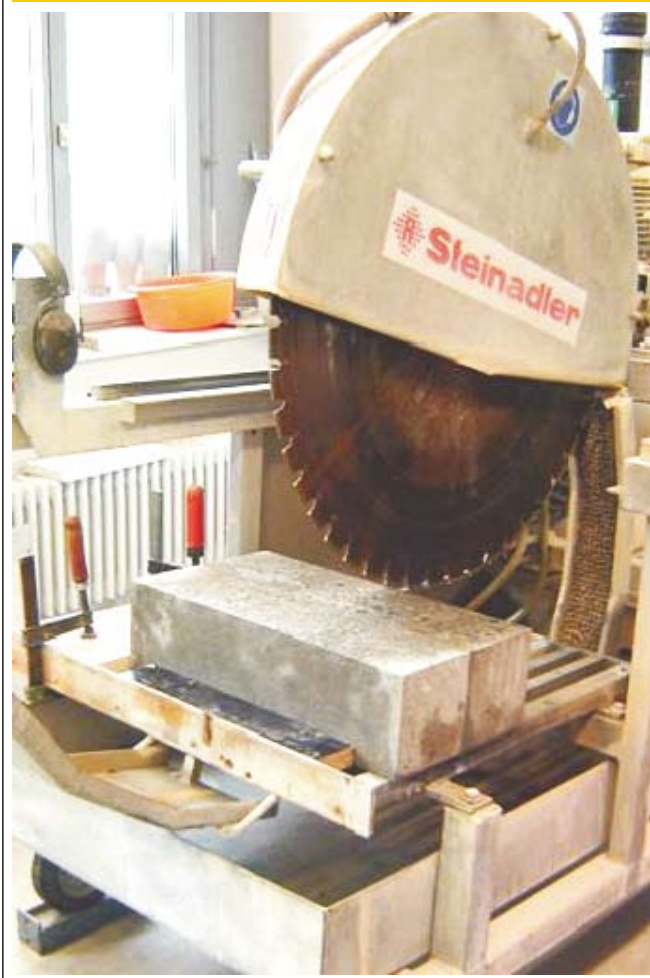
Figure 5 – Device used to notch the concrete beams
