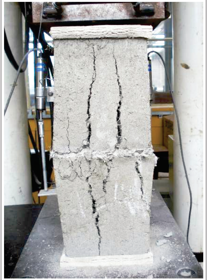
Figure 12 – Ductile break of the prisms with the added fiber
