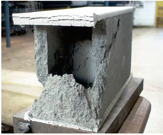
Figure 10 –Fragile break of the blocks without the added fiber
