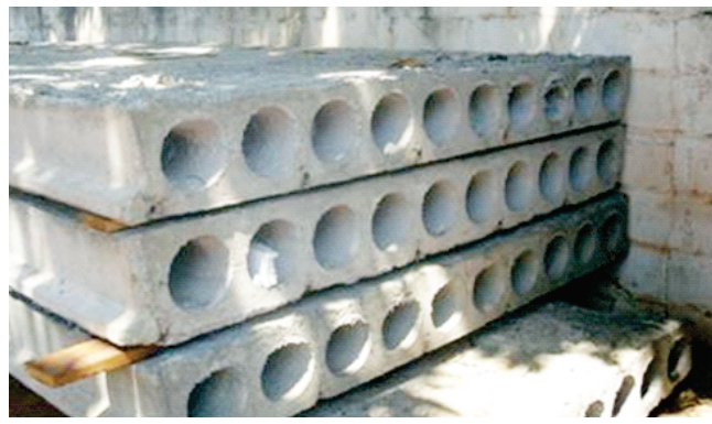
Figure 12 – Hollow core slabs used in the test and manufactured by LATTICE SLAB (LAJE TRELIÇADA) IND. and COM. LTDA
