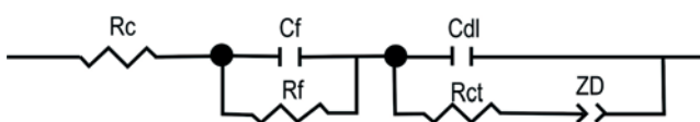
Figure 4 – Equivalent circuit for concrete proposed by John et al. (6). R_c : concrete strength; R_f and C_f : resistance and capacitance of the film; Z_d : diffusion impedance; R_{ct} and C_{dl} : charge transfer resistance and double layer capacitance
