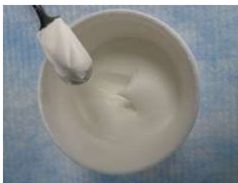
Figure 1: \beta -TCP ink consistence. Notice the stiff peak formed once a spatula is pulled straight up out of the ink.
