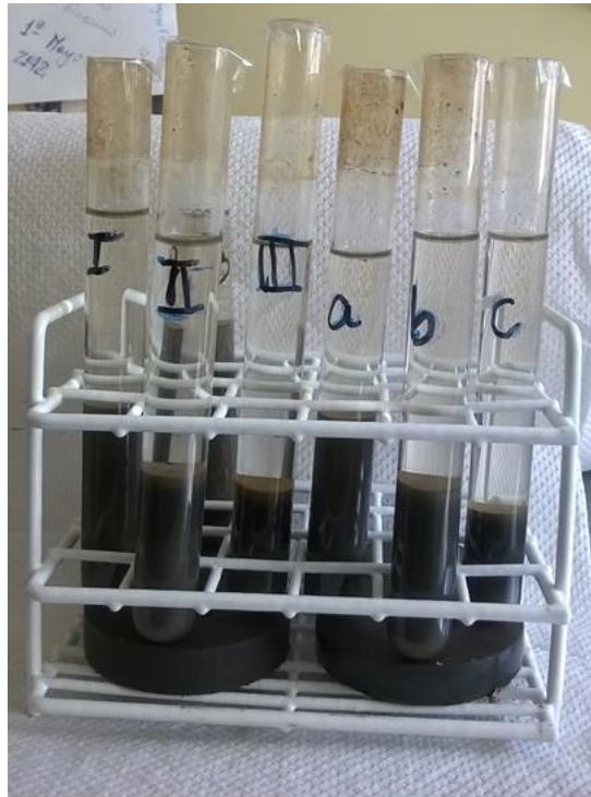
Figure 4: Demulsification after six months (magnetically assisted).
