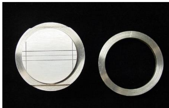
Figure 1: Stainless-steel die (ISO 21563:2013 and 4823:2015).
