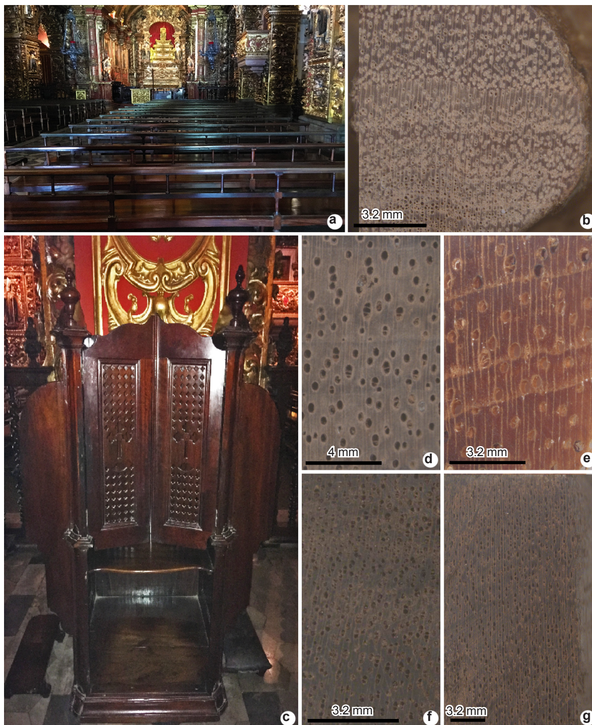
Figure 3 – a. Pew. b. Macroscopic anatomical characteristics of Paratecoma peroba ( peroba-do-campo ). c. Confessional. d. Macroscopic anatomical characteristics of Tachigali sp. ( tachi ). e. Macroscopic anatomical characteristics of Cedrela sp. ( cedro ). f. Macroscopic anatomical characteristics of Ocotea sp. ( imbuia ). g. Macroscopic anatomical characteristics of Nectandra sp. ( canela ).
