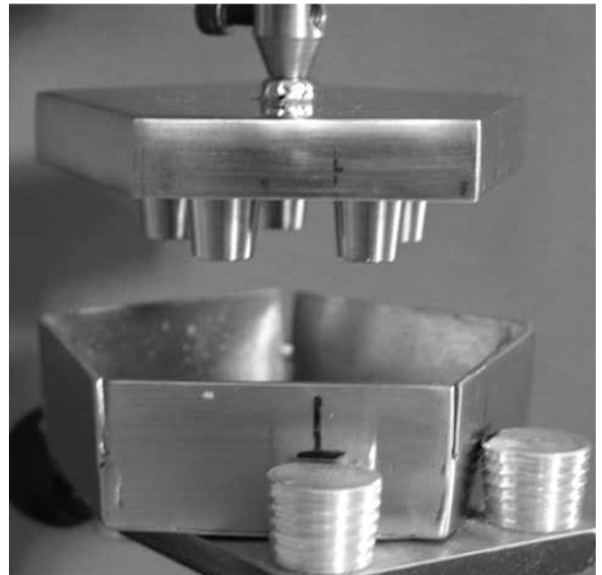
Figure 1. Moulding set/matrix positioned in the liner.
