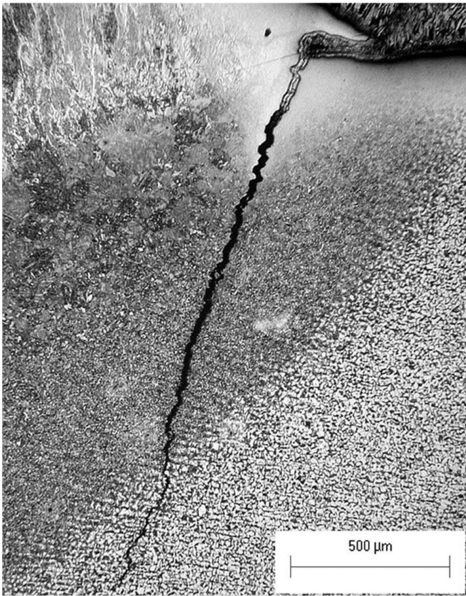
Figure 9. Crack initiation and propagation.
