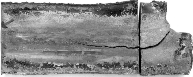
Figure 7. Crack in zinc coated welded steel structure.
