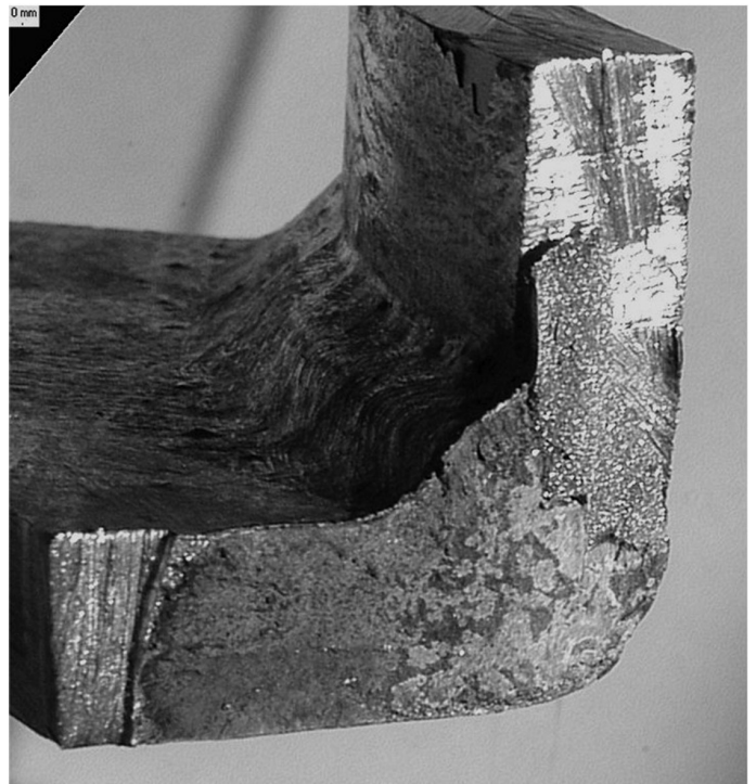
Figure 6. Crack morphology in a circumferential weld between the plate and tube.
