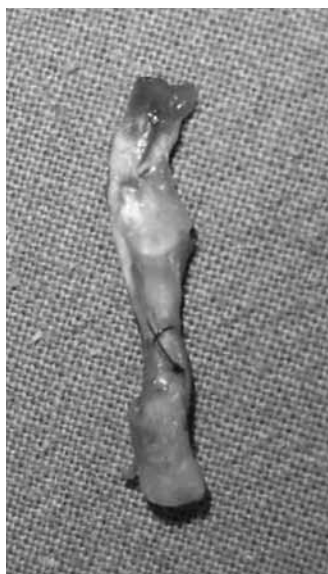
Figure 3 – Isolation of the calcaneal tendon of the rat with the suture stitch before the biomechanical test.
