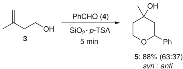
Scheme 2. Synthesis of model compound 5 .
