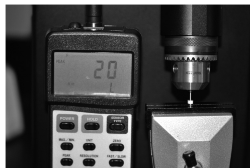
Figure 2. Torque application; implant was positioned in a vise grip, and the digital torque wrench was used to apply a 20 Ncm torque.
